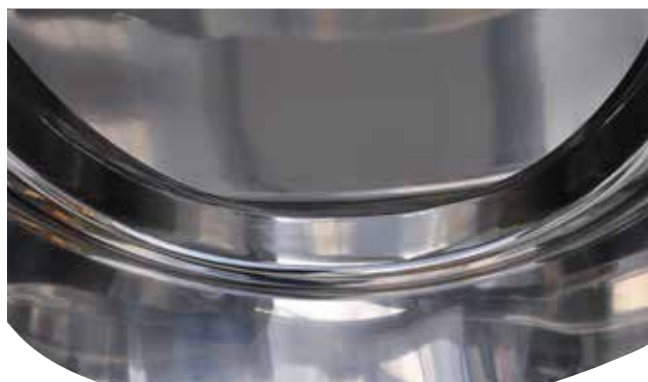
Trimmed and polished interior welding of round hatch
